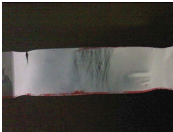
Figure 4 Exhibition of stress whitening and necking in the 4 pph PLA nanocomposite. [Color figure can be viewed in the online issue, which is available at www.interscience.wiley.com .]
